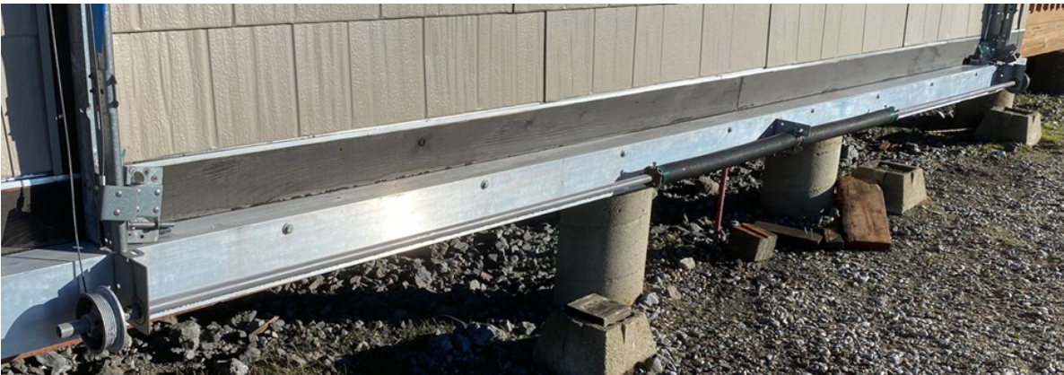
The redesigned axle assembly mounted on a 20' aluminum beam
